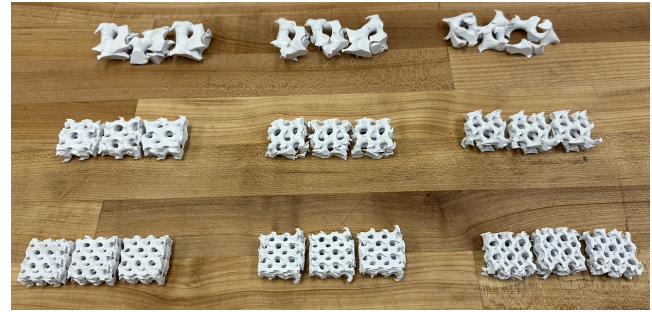
Figure 6: The 27 crushed gyroids after testing.
